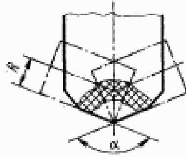
$\alpha = 136^\circ;$<br>$R = 2 \text{ мм} — \text{радиус цилиндра}$ |
